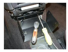
Attach support bracket for stout console (#2) to vehicle and to frame support bracket using OEM hardware and #10 x ½" phillips machine screws and washers
